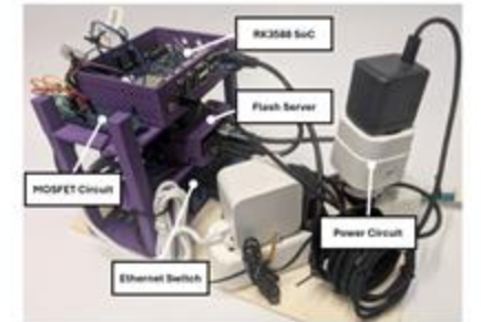
Figure 1. OPENCCA tooling. The RK3588 connects over ethernet to a flash server (Raspberry Pi). It controls a MOSFET and power circuit to flash new firmware and exposes UART access.
